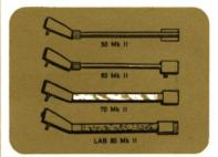
The epitome of low mass tone arm construction is the exceptional arm of the Lab 80. It is made of Afrormosia – the least resonant of woods...therefore, ideal for this special application. The wooden shaft is rigidly held by a "T" of aluminum... an ingenious combination of materials promoting flawless tracking performance.
