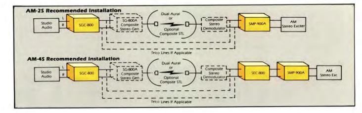
**SEC-800**: The SEC-800 SPECTRAL ENERGY COMPRESSOR is a musical sounding four band compressor/limiter featured in the AM-4 system and may be added to existing AM-2 systems.
