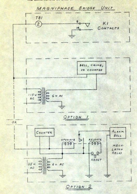
CONTINENTAL ELECTRONICS MANUFACTURING CO. REVISIONS DATE APP USED WITH 19876-B DALLAS, TEXAS **STEAM POWERED RADIO.COM** MAGNIPHASE MATL EXTERNAL ALARM CIRCUIT UNLESS OTHERWISE SPECIFIED SCALE: DIMENSIONS IN INCHES 19939-A PAS ENG. APP'D. TOLERANCES FRACT. DEC. ±1/2° 7-11-59 ± /64 ±.015
