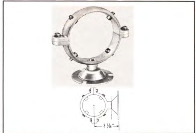
TYPE NO. 211-835 (NPN) — Hanger, slip type, flange mount supports transmission indoors or outdoors. Permits expansion. Weight: 1 1/2 lbs.
