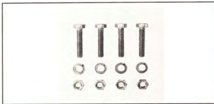
TYPE NO. 315-825 (NPN) — Hardware set for 1\frac{5}{8} " flanges. Consists of 4 ea. stainless steel bolts, nuts and lockwashers, \frac{5}{16} "-18 x 1\frac{1}{2} " lg. Weight: 3\frac{1}{2} oz.
