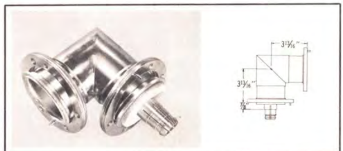
TYPE NO. 494-835 (Part No. 097 6986 —) — Elbow assembly, miter, 90 degree, male-female, reinforced, swivel flanged. Includes one affixed male anchor insulator-connector, "O" ring and hardware. Weight: 7 lbs. 12 oz.
