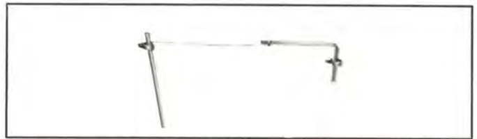
Type No. 50-150 ASSEMBLY for grounding 7/8" Spir-O-line at base of tower; Copper ground rod is 1/2" dia. and 6 feet long, copper wire is #10 AWG and 10 feet long. (NPN).
