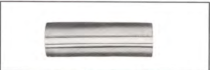
Type No. 93-500 MOUNTING SLEEVE, split, 1/2" size, used when fastening plain cable with wraplock to tower leg. (NPN).
