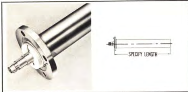
TYPE NO. 105-825 (NPN) — Line assembly, length to be specified, flanged one end. Includes anchor insulator-connector assembly, "O" ring and hardware. Weight: 1 lb. 3 1/2 oz. + 1 lb. 3 oz./ft.
