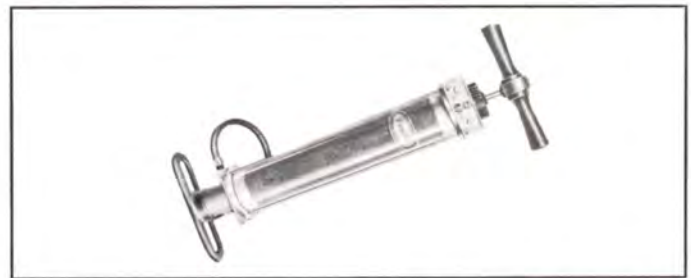
Type No. 30-150 DEHYDRATOR, hand pump consists of blue indicating gel, and will pressurize up to 1000 ft. of 7/8" or 250 ft. of 1 5/8" Spir-O-line. (Part No. 099 0517 00).
