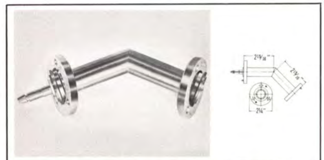
TYPE NO. 448-815 (NPN) — Elbow assembly, miter, 45 degree, swivel flanged, male-female. Includes one anchor insulator-connector, "O" ring and hardware. Weight: 1 lb. 1 oz.
