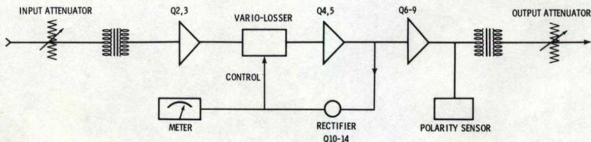
Figure 4-1. Volumax - Block Diagram
