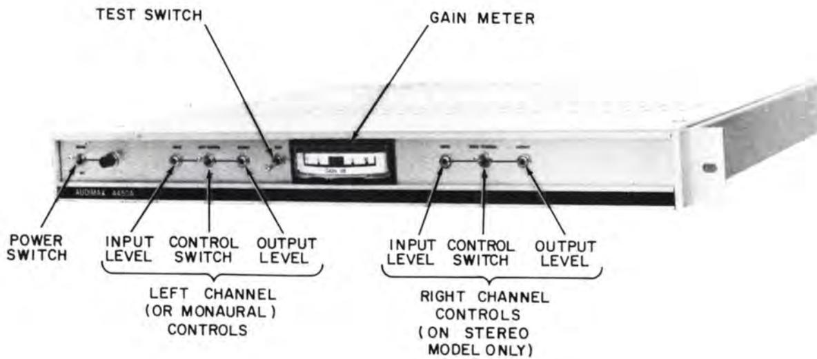
Figure 3-1. Audimax Unit, Front Panel Controls
