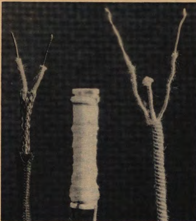
CABLE BALANCING CAPACITANCES—OLDER TYPE SHIELDED TWISTED PAIR AT LEFT—NEWER TYPE SPIRALLY WOUND PAIR AT RIGHT—UNIT USED AT END OF REPEATER SECTION IN CENTER
