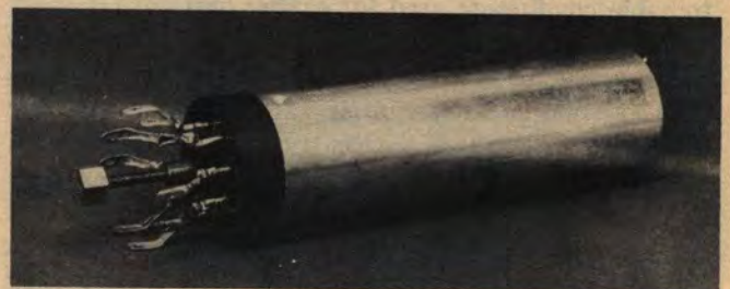
CONSTRUCTION OF CROSSTALK BALANCING COIL
