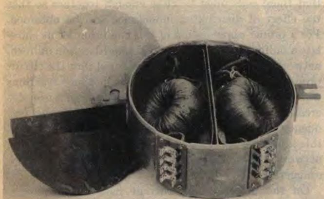
PHANTOM LOADING COILS FOR TOLL ENTRANCE CABLE ASSEMBLED IN SHIELDED CASE TO PREVENT CARRIER CROSSTALK
