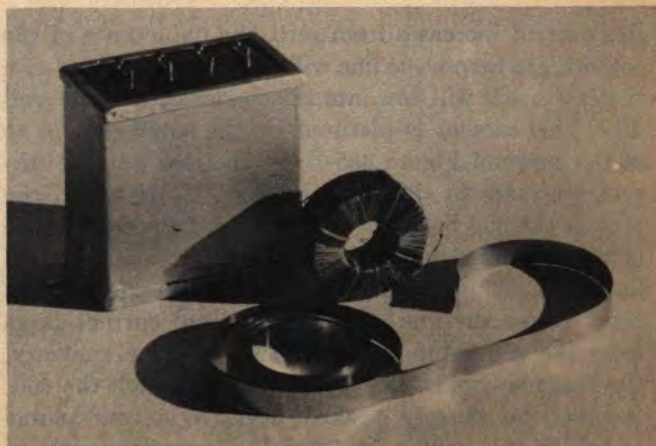
HARMONIC PRODUCER COIL SHOWING PERMALLOY TAPE CORE
