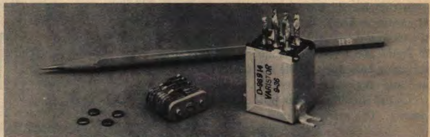
COPPER-OXIDE VARISTOR UNIT USED AS MODULATOR AND DEMODULATOR
