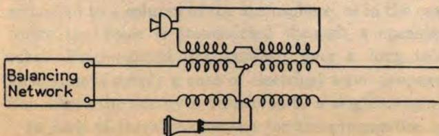
FIG. 250. THE HYBRID COIL
