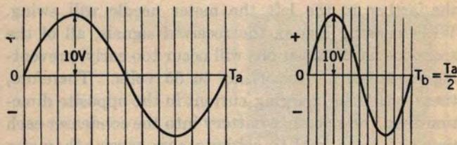
FIG. 194. SINE WAVES OF DIFFERENT FREQUENCY
