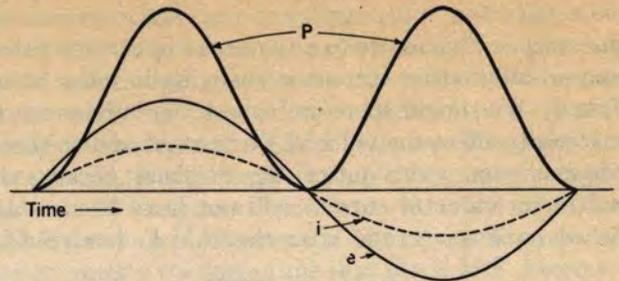
FIG. 203. POWER IN A.C. CIRCUIT WHEN CURRENT AND VOLTAGE ARE IN PHASE
