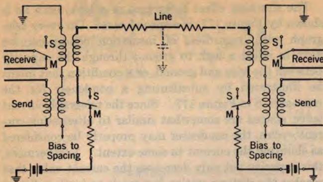
FIG. 180. NEUTRAL TELEGRAPH CIRCUIT EMPLOYING BIASED RELAYS
