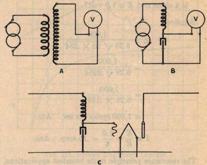
FIG. 231. USE OF RESONANCE PRINCIPLE TO INCREASE VOLTAGE
