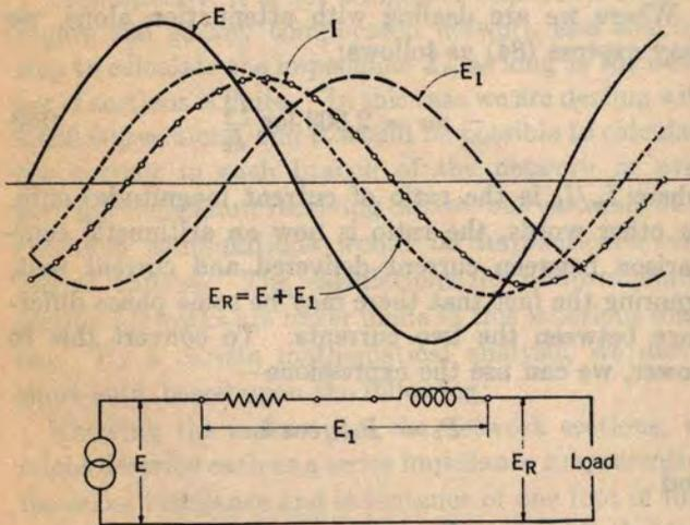
FIG. 264. VOLTAGES AND CURRENT IN AN INDUCTIVE CIRCUIT
