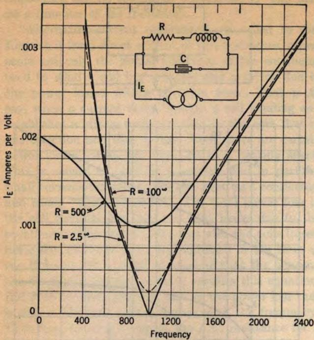
FIG. 230. CURVES OF CURRENT VALUES IN ANTI-RESONANT CIRCUIT
