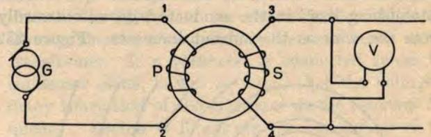
FIG. 235. ELEMENTARY TRANSFORMER CIRCUIT
