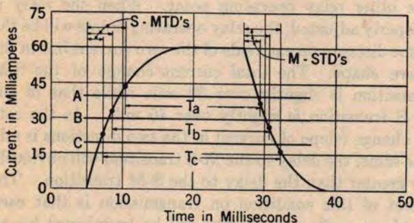
FIG. 182. EFFECT OF RELAY BIASING CURRENT ON SIGNAL LENGTH
