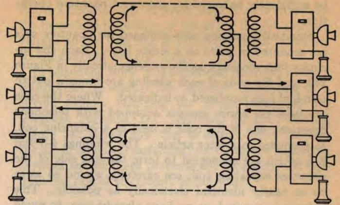
FIG. 239. PRINCIPLE OF THE PHANTOM CIRCUIT
