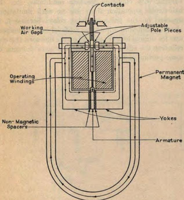
FIG. 155. MAGNETIC CIRCUIT OF THE DIFFERENTIAL POLAR RELAY
