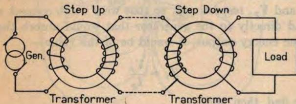
FIG. 237. USE OF TRANSFORMERS IN POWER CIRCUIT
