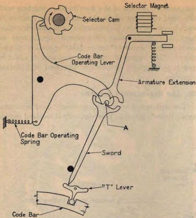
FIG. 170. RECEIVING MECHANISM OF SINGLE MAGNET TELETYPEWRITER
