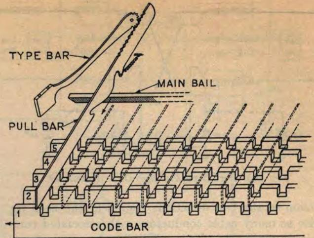
FIG. 168. SELECTING MECHANISM OF RECEIVING MACHINE
