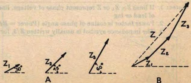
FIG. 222. GRAPHICAL ADDITION OF IMPEDANCE VECTORS
