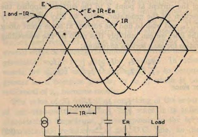
FIG. 265. VOLTAGES AND CURRENT IN A CAPACITIVE CIRCUIT
