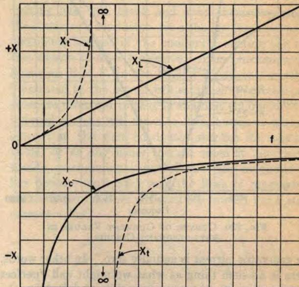
FIG. 229. ANTI-RESONANT CIRCUIT
