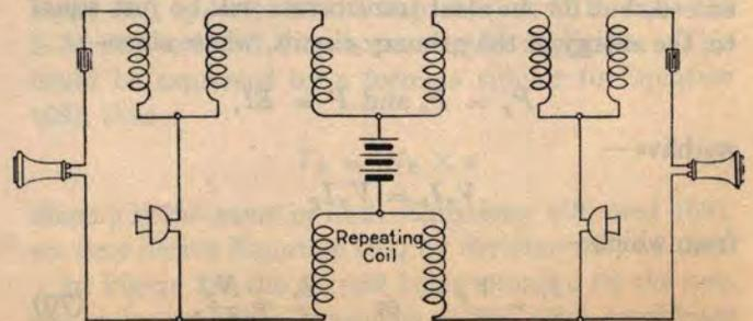
FIG. 238. TRANSFORMERS IN COMMON BATTERY TELEPHONE CONNECTION
