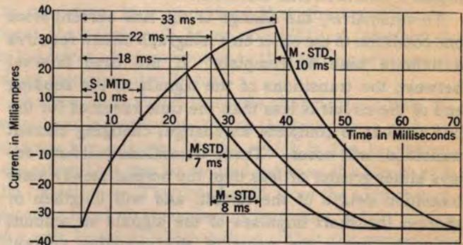
FIG. 187. CHARACTERISTIC DISTORTION EFFECTS ON SIGNAL LENGTHS AT 40, 60, AND 75 SPEED OPERATION
