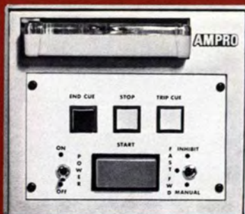
AMPRO SERIES CT 2500 is available as a reproducer for NAB Type A and AA cartridges — monaural and stereo.
