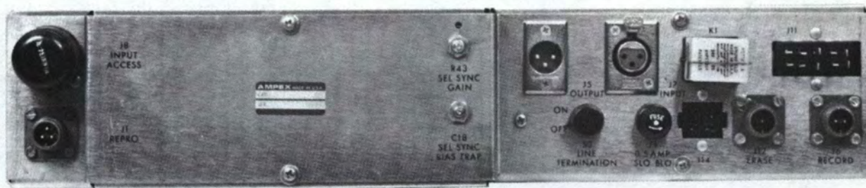
Fig. 2-4. Record/Reproduce Unit (Rear)
