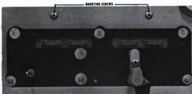
4A-2. Head Cable Box
