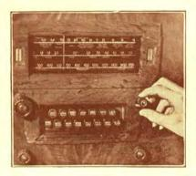
3. Grasp this set-up knob and pull it out AS FAR AS IT WILL GO "rocking" it slightly at the same time so that the gears in the mechanism at the rear will mesh properly.
