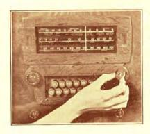
6. Grasp the set-up knob again and tune the receiver to the desired station. TUNE CAREFULLY AND WATCH THE VISUAL TUNING INDICATOR FOR THE POINT OF MINIMUM ILLUMINATION SO THAT THE RECEIVER WILL BE CORRECTLY TUNED TO THE STATION.
