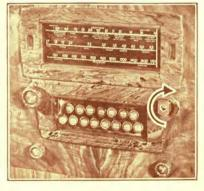
5. Push any button you wish to set up for a station. There need be no relationship between the position of the button on the keyboard and the station on the dial. Be sure the button is pushed all the way in. You will note that as the button is pushed in, the word "Automatic" will appear illuminated on the small indicator at the right side of the dial, and the keyboard mechanism will in-
