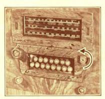
II. Then turn the set-up knob to the LEFT (counter clockwise). The knob will turn rather stiffly and the dial pointer will travel over to the extreme left side of the dial scale. CONTINUE TO TURN THE SET-UP KNOB TO THE LEFT even after the pointer reaches the end of the dial scale. APPLY A FIRM PRESSURE UNTIL THE KNOB REACHES A DEFINITE STOP.
