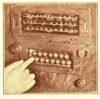
stantly move the station indicator to some position on the dial scale, depending upon the previous setting of the mechanism. This need have no relation, however to the station for which you desire to set the button.
