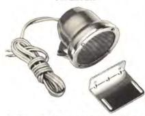
Handles up to 20 watts of audio power, with frequency range 3000 to 17000 CPS, Built-in crossover network. Mounting bracket with 2 mounting holes is attached. Metallic grey finish housing, 3-ft, twin rubber covered cord is included. Extra vertical adjustable bracket suitable for flush mounting against baffle supplied complete with hardware. Voice coil impedance 16 ohms. Size  $2^{3}\!\!/\!\!4''$  dia. x  $2^{1}\!\!/\!\!4''$ deep, Individually boxed.
