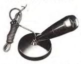
Desk type, omni-directional. Suitable for tape recording voice, instrumentalists, and broadcasting, public address etc. Supplied with swivel base desk stand, adaptor for 5/8" -27 thread for floor stand and 8 foot plastic covered microphone cable. Base has rubber ring to protect table surfaces.
