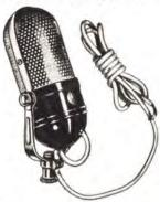
Omni-directional studio type crystal microphone, suitable for conference groups, PA, tape recordings, etc. Dual phased crystal units, vertically mounted. Mounting thread 5/8"-27. Supplied with 4 feet plastic covered microphone cable.
