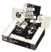
The entire unit is assembled on a plywood base, and clasp holders are provided for two flashlight cells to supply operating voltage of 3 volts. Ordinary 11/2 Volt Flashlight cells are used.
