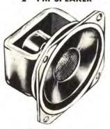
2" x 2" x 11/8", overall size. 15/8" square mounting centers. .5 oz. alnico V magnet. 8 ohm voice coil, 100 milliwatt power rating. Ideal for miniaturized transistor applications and as a super tweeter for Hi-Fi speaker systems.
