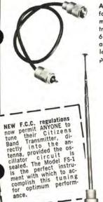
ATTENTION "HAMS" - Use the FS-1 "stock" for Field strength measurements of your 10 meter rig, just by retuning the antenna trimmer. The unit can also be used for 2 and 6 meters by a simple change of capacitor and collapsing of whip antenna to proper length. Load box can be used for short periods up to 10 watts for mobile rigs.
