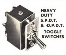
Bat handle, plastic case. Supplied with very attractive red and black "on-off" plate. Rated 10 amps 125 volts, 5 amps 250 volts. Mounting centers 156". 3/16" shank.
