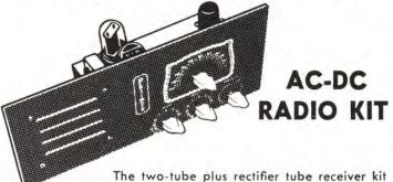
is more elaborate than the one-tube and much greater in signal strength—permitting use of a 4" P.M. speaker.
