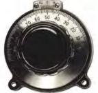
Smooth friction vernier drive dials, with clearly etched numerals on professional-finish satin background, Calibrated over 180° reading from 0 to maximum setting by clockwise rotation. Planetary drive with 8 to 1 ratio. Precision brass and bronze parts are mounted in attractive black phenolic housing. Furnished with matching black phenolic knob. Surface mounting for  $\frac{1}{4}$ " shaft.
