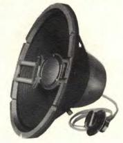
A 12 inch coaxial speaker with dual tweeters mounted before the woofer at opposing angles to project highs over a broad angle. Heavily constructed on a die cast aluminum frame.
