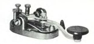
STANDARD PRECISION-BUILT TELEGRAPH KEY with smooth, velvet action for code practice and use with transmitters. Eight ball bearings supporting the key are completely adjustable for friction. Contacts are 1/8" pure silver and are also easily adjustable for contact spacing and tension, Heavy brass base is drilled for easy mounting.
