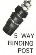
Rugged plastic body with a banana plug receptacle and solder connections on base. Has a non-removable head and a wire hole through post. Rated 2,000 volts; 30 amps. Mounts through 1/2" panel hole. Overall length: 1 3/4". Choice of red or black. Please specify color.
