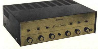
All of the latest engineering features combined in one compact unit to deliver clean amplification of fine sound. Delivers 30 watts of music power per channel for a 60 watt total. Response from 20 to 50,000 cps  $\pm 0.5$  db.; with a 9 tube-2 diode, push-pull, fixed bias circuitry. Contained in a smart metal cabinet with brushed-gold face plate. 153/4" wide, 5" high, 124/2" deep.
